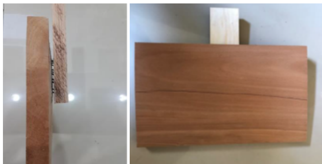
Fig. 12. Failure modes of the joints: a) separation from connection points; b) main member rupture
