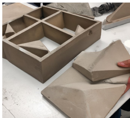
Fig. 2. Wall cladding element in realization – the panels of chamotte clay (photo by A. Bonenberg)
