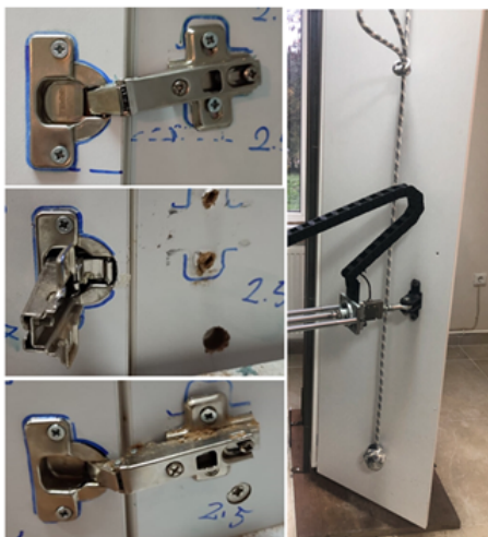
Fig. 5. Three-hinged MDF door after test
