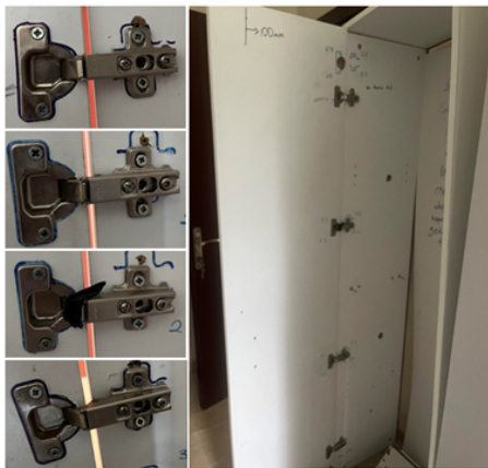
Fig. 7. Four-hinged MDF door after test
