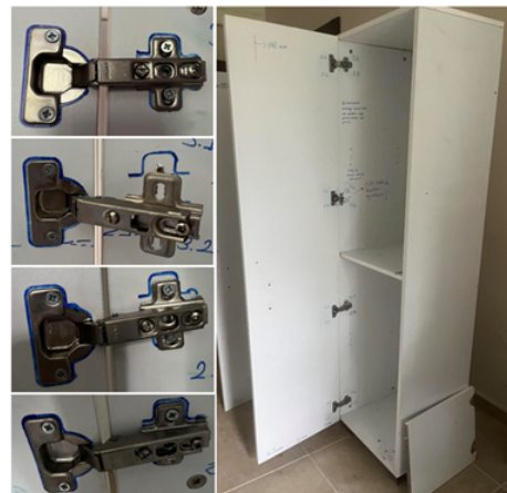
Fig. 8. Four-hinged PB door after test
